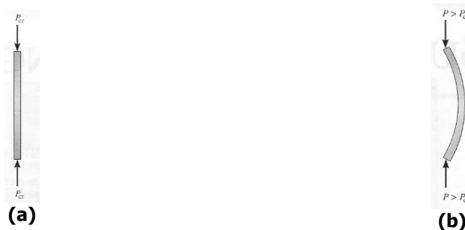
Figure 1.- Definition of the structural element known as column (R.C. Hibbeler, 2011) (a) The column does not suffer buckling if P=P_{cr} . (b) The column suffers buckling when P>P_{cr} .
